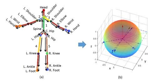
Fig. 2. (a) A skeleton and its joints. The C. Hip is the root of the kinematics chains formed by joints (marked by arrows). (b) An illustration for the skeleton feature computation. For better visualization, only 5 joints are shown in the unit sphere.
